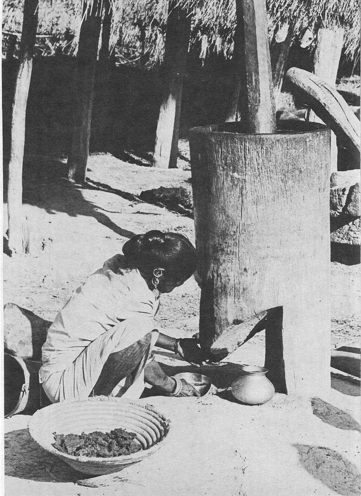
Collecting the oil as it is pressed out of the kolh .
