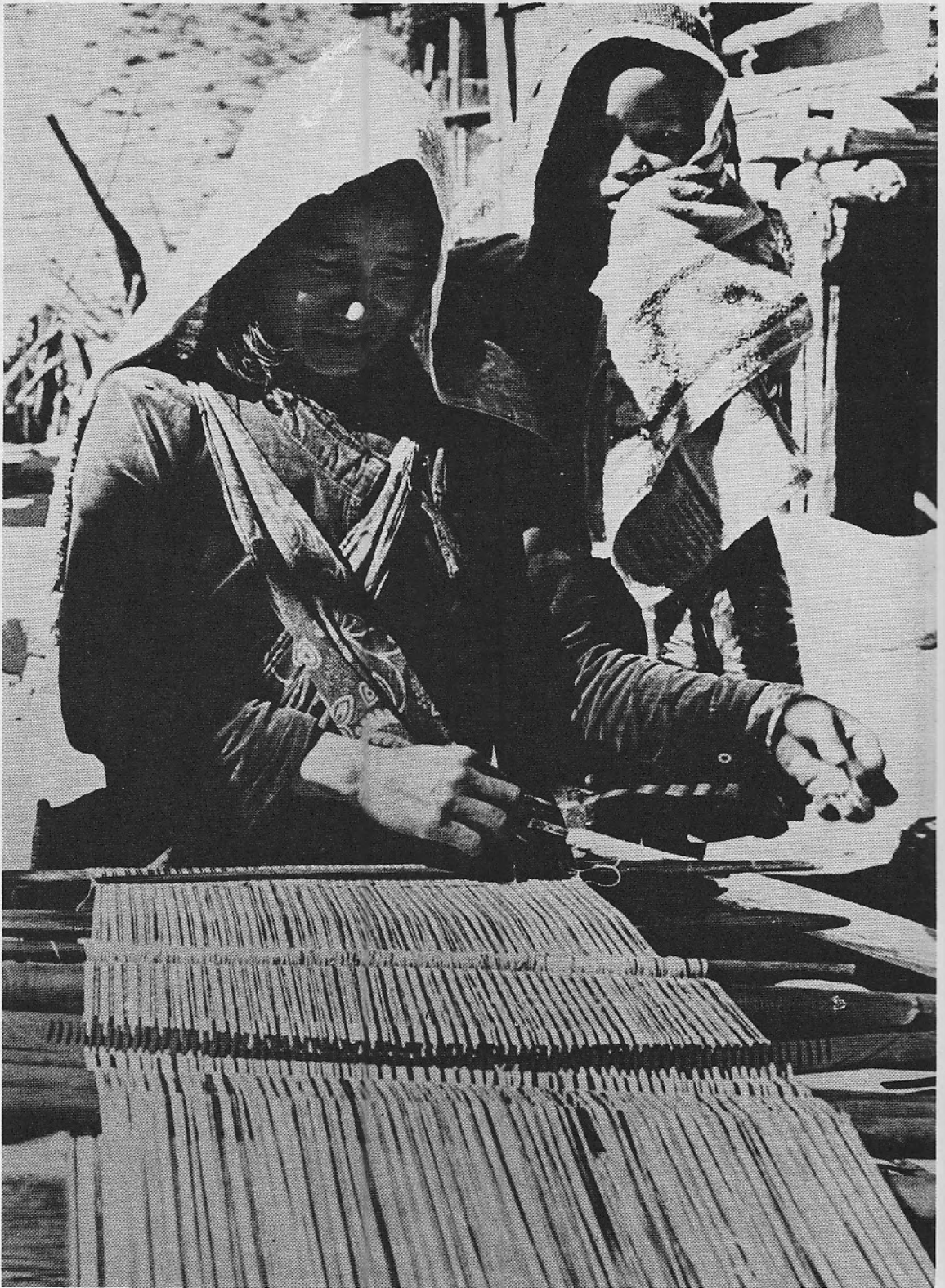
A woman weaving cotton cloth on a backstrap loom in her courtyard.
