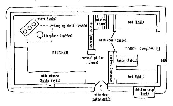
Fig. 5.1 Ground Floor Plan of Yakha House
