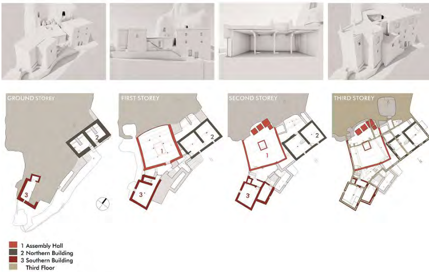
Fig. 9 — Building phases of Dangkhar's main building. TU Graz 2013.
