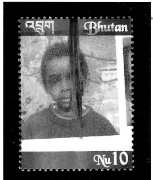
Typical error from the old printer on personalized stamps showing misplacement and the running black ink
