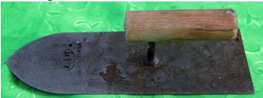
Photo 243. G.yos this are used to pave and smooth mud and cement on walls and the ground.
