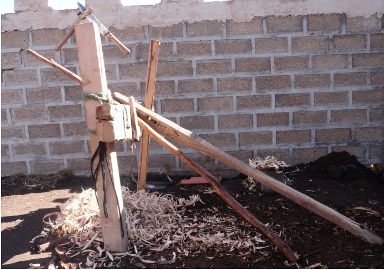
Figure 9. The 'u cur ha is used to straighten yurt poles.
