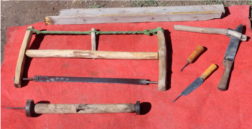
Figure 6. Yurt-making tools. The piece of wood at the top is the gcur shing . It is part of the ' u cur ha ' and is used to straighten the yurt poles. The knife and stick below it on the right are also part of the ' ur cur ha '. A saw is to the left. Other tools are drills.
